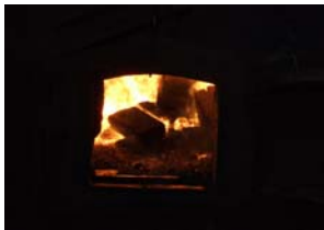
Figure 4: press cake in burner (picture:J.van Eijck)
